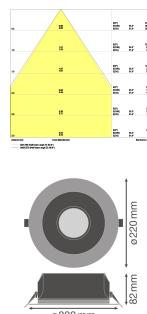
**Scheda tecnica Ledvance Downlight LED Performance DN195 21W 2520lm 65D - 840 Bianco Freddo | 220mm - IP54**
